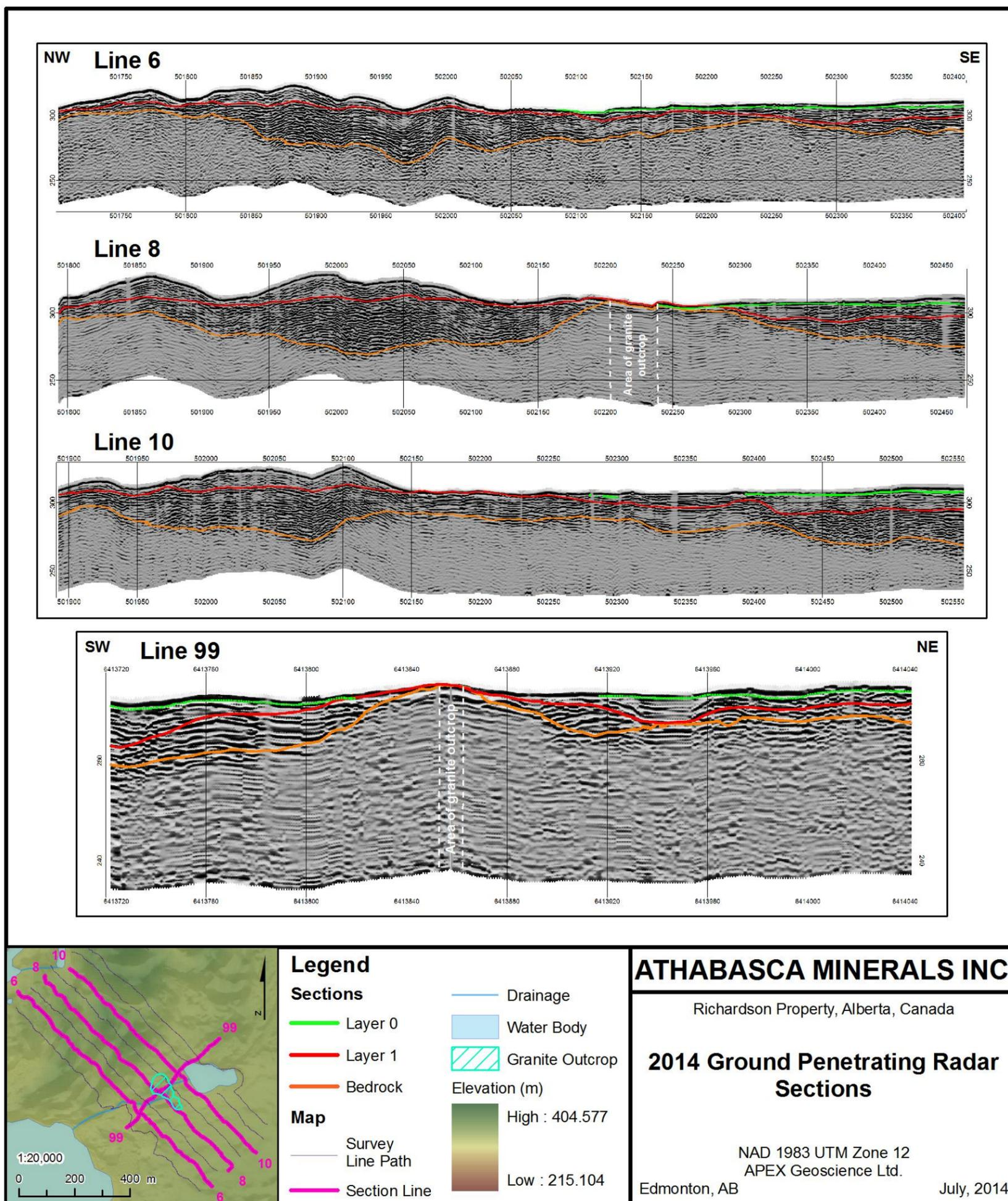
Figure 12. Gridded Ground Penetrating Radar responses to the top of the “Layer 1” reflector (or top of Winnipegosis Formation).
