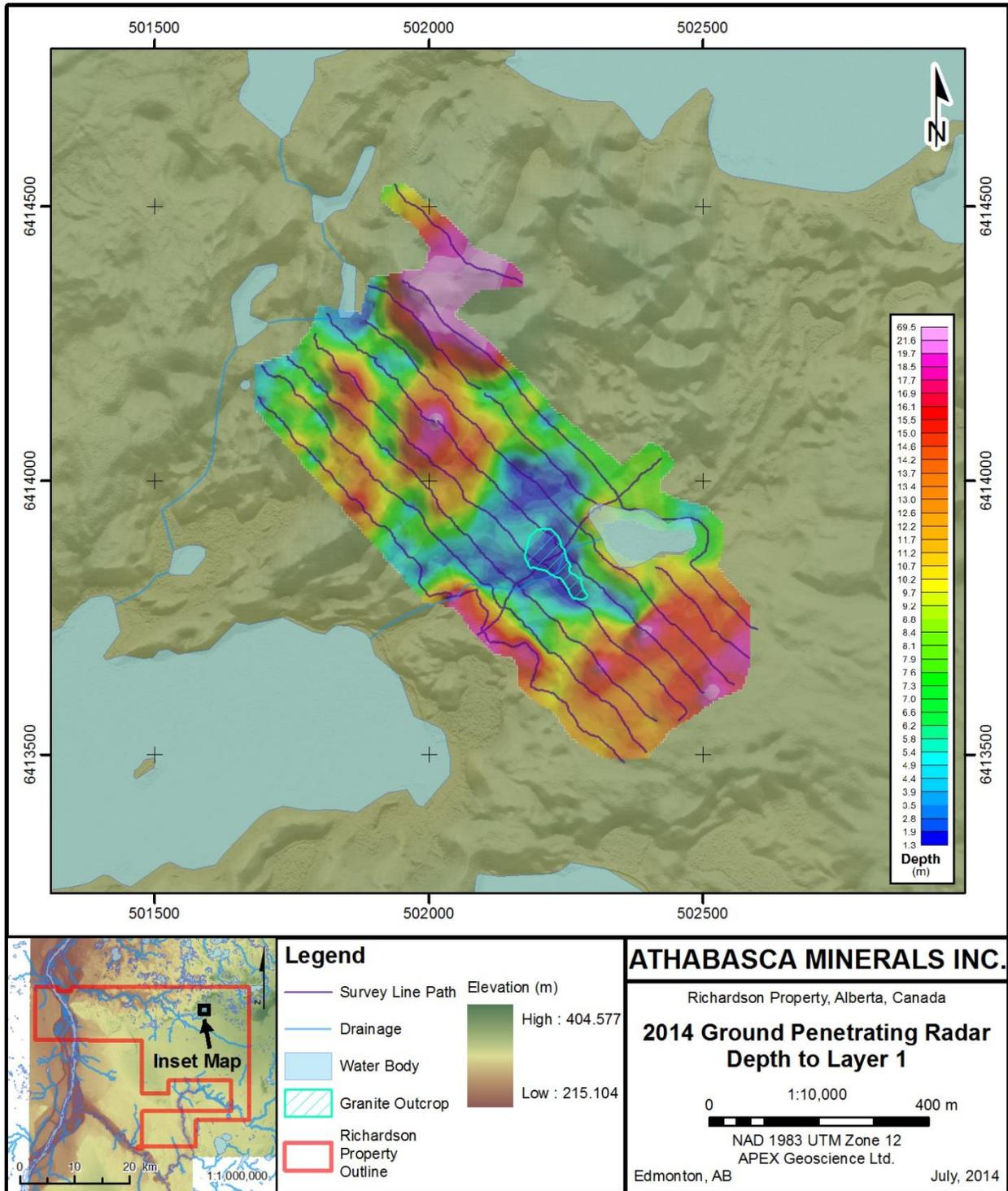
Figure 13. Gridded Ground Penetrating Radar responses to the top of the “Bedrock” reflector (or top of the Precambrian basement granite).
