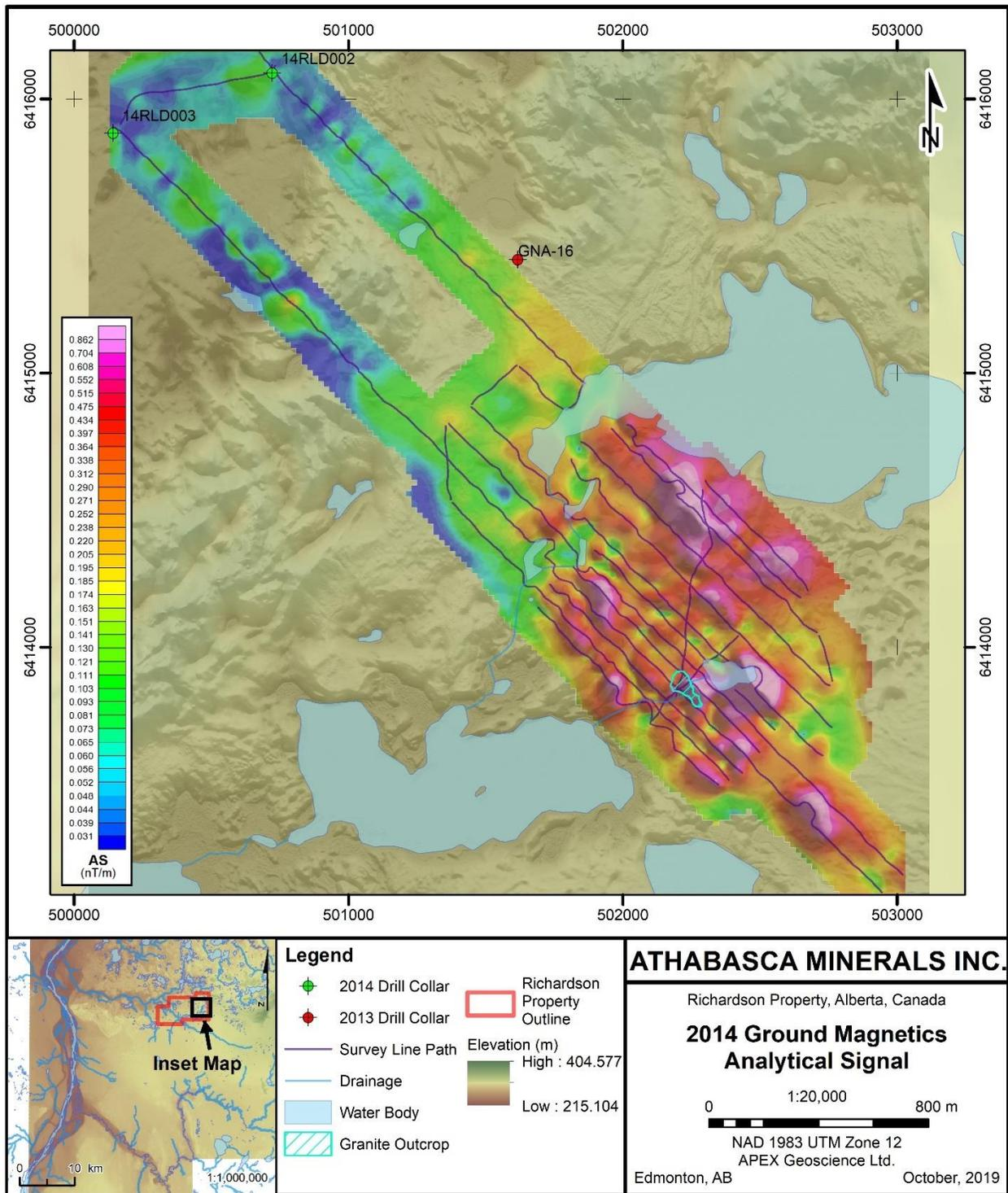
The ground magnetics survey data highlights three distinct litho-magnetic zones at the Richardson Property geophysical survey area (e.g., Figure 16), including:
